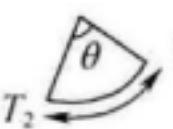
$$T_2 = T_{1e^{\mu\theta}} - 9.8WR[2\sin\theta + (1 + \mu^2)/\mu(e^{\mu\theta} - \cos\theta)]/(1 + \mu^2) \quad (\text{A. 0. 5-4})$$
